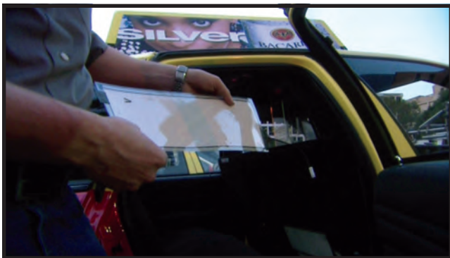
1.4 One of the ELD panels specially made for illuminating the cab interior.
