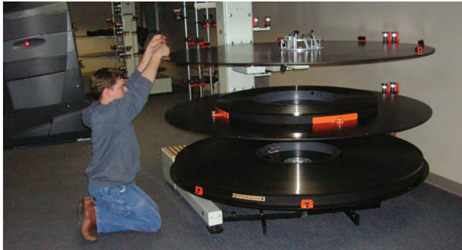
1.14 Most multiscreen theaters use platter projection, which winds the film in long strips and feeds it to a projector (seen in the left rear). The film on the platters is an Imax 70mm print.
